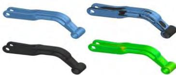
Figure 10. Reverse engineering on a lever
