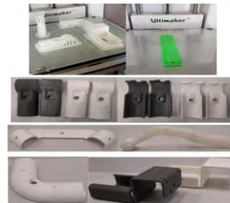
Figure 6. Scanned elements made with 3D printing technology
