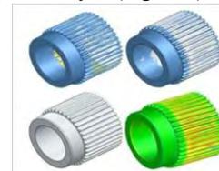
Figure 7. Scanned pulley, 3D model of the pulley and deviation display
