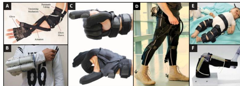
Selection of indicative wearable soft robotic solutions that utilize fluidic and cable driven principles of operation to assist individual biological joints with motion of: (A) the wrist (N. W. Bartlett, 2015), (B) the elbow (T. Noritsugu, 2008), (C) the hand (P. Polygerinos, 2015), and (D-F) the legs (M. Wehner, 2013, K. Subramanyam, 2015, Y.-L. Park, 2014).
