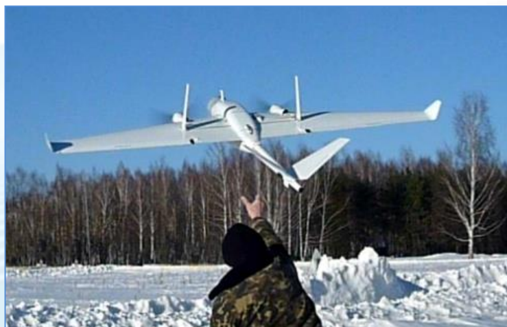
Take-off by hand (UAV “Busel M40”)
