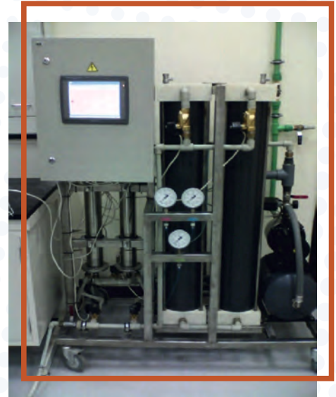
Automated microfiltration water purification unit (in cooperation with the Institute of Chemistry of New Materials)
