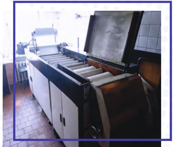
Pilot plant for manufacturing of substrate-reinforced membranes
