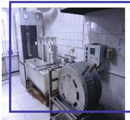
Equipment set for manufacturing of capillary membranes
