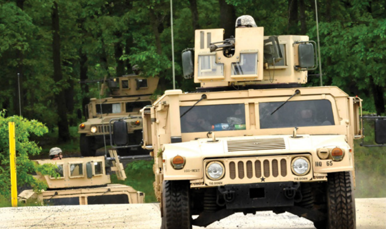
Figure 18. A Ricardo Defense Systems pilot project retrofitted 10 Michigan National Guard vehicles with antilock braking systems and electronic stability controls to reduce high mobility multipurpose wheeled vehicle fatal rollovers. Credit: Department of Defense
